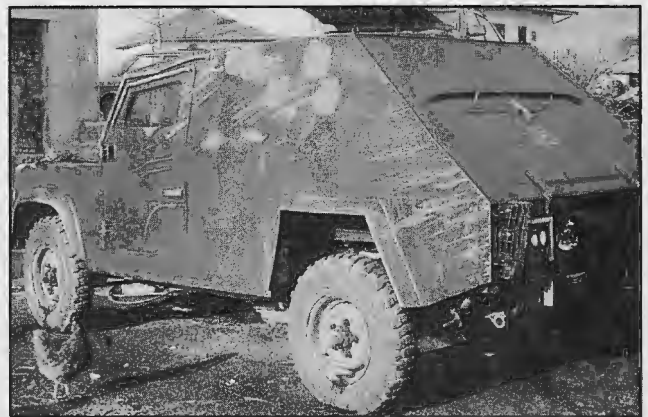
Bullet-scarred ITN armored Land-Rover was custom built in England for use in Africa. Bullet strikes are probably from 7.62x39mm and/or 7.92mm M76 sniper rifle rounds. Photo: Chuck Fremont
